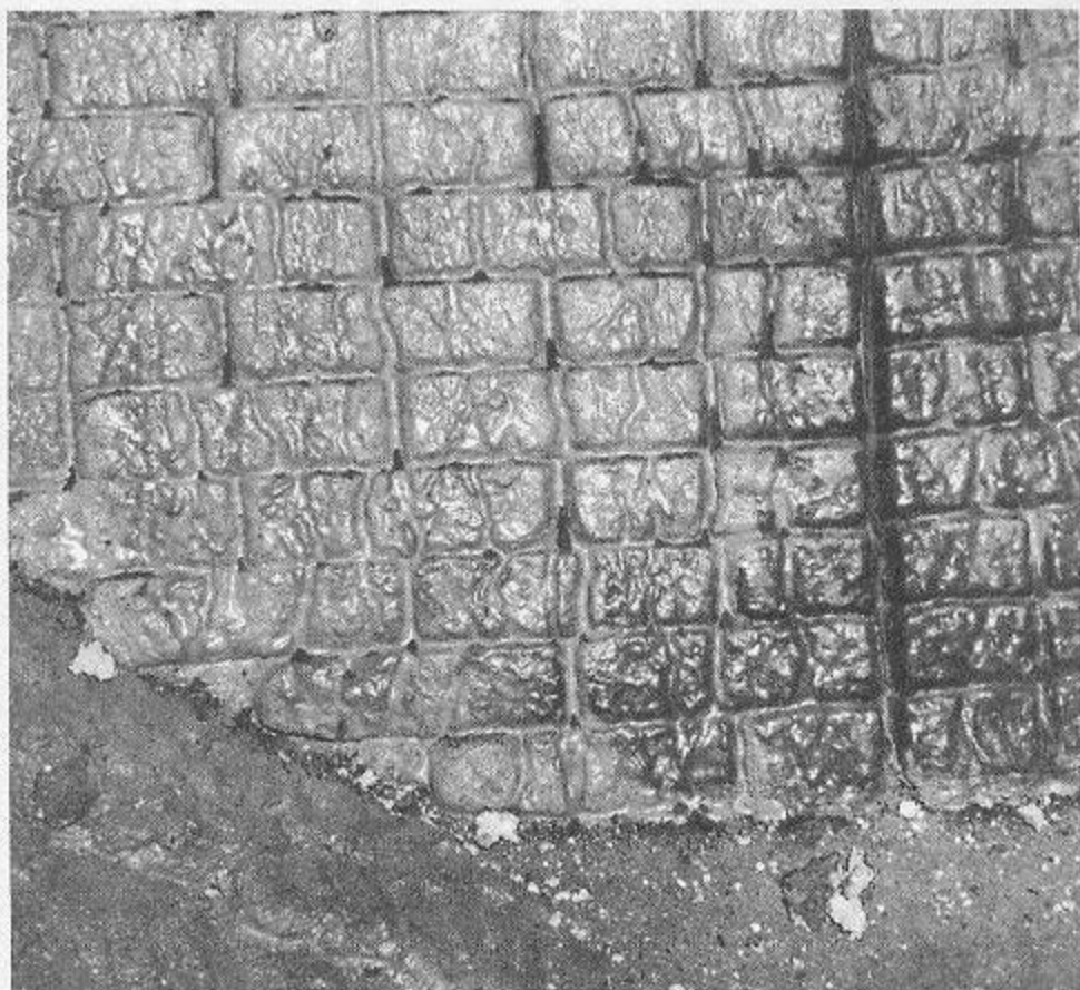
Figure 2-40.—Glassy slag resulting from sea water contamination of fuel oil.
