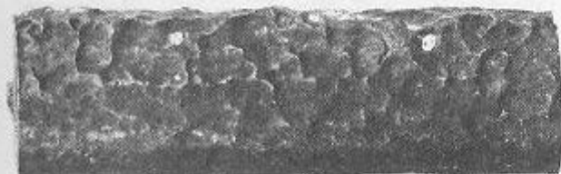
Figure 2-19.—General fireside thinning of stainless steel superheater tube (result of fuel ash damage).
