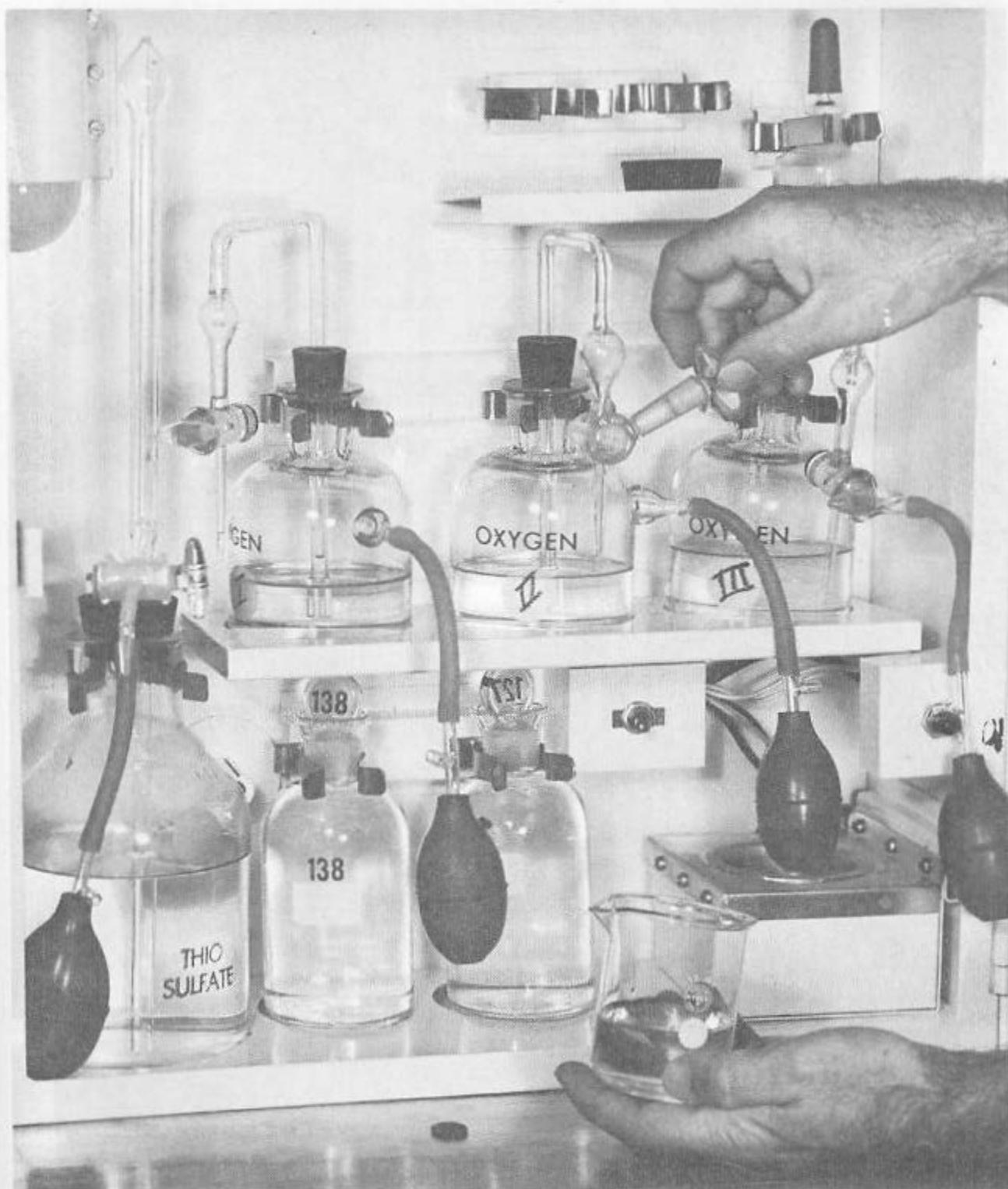
Figure 4-34.—Replacing the plug in the stopcock of the OXYGEN II pipette (dissolved oxygen test).
