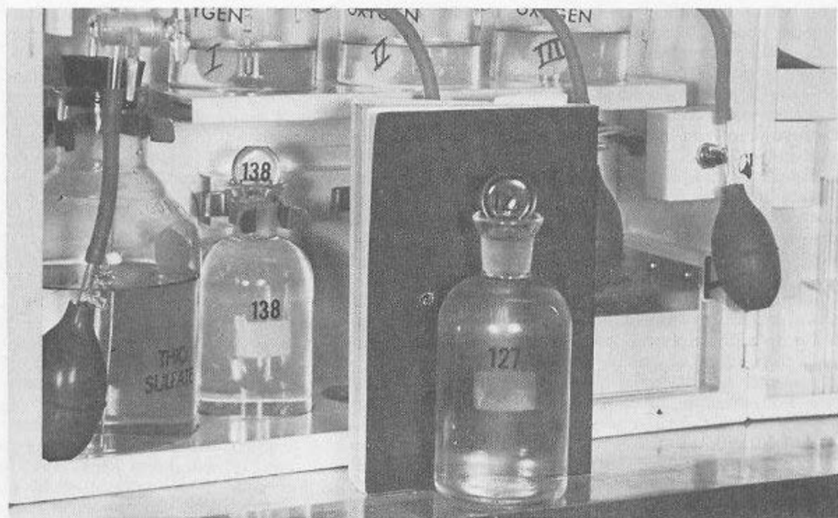
Figure 4-41.—Adding OXYGEN III solution to the sample (dissolved oxygen test).
