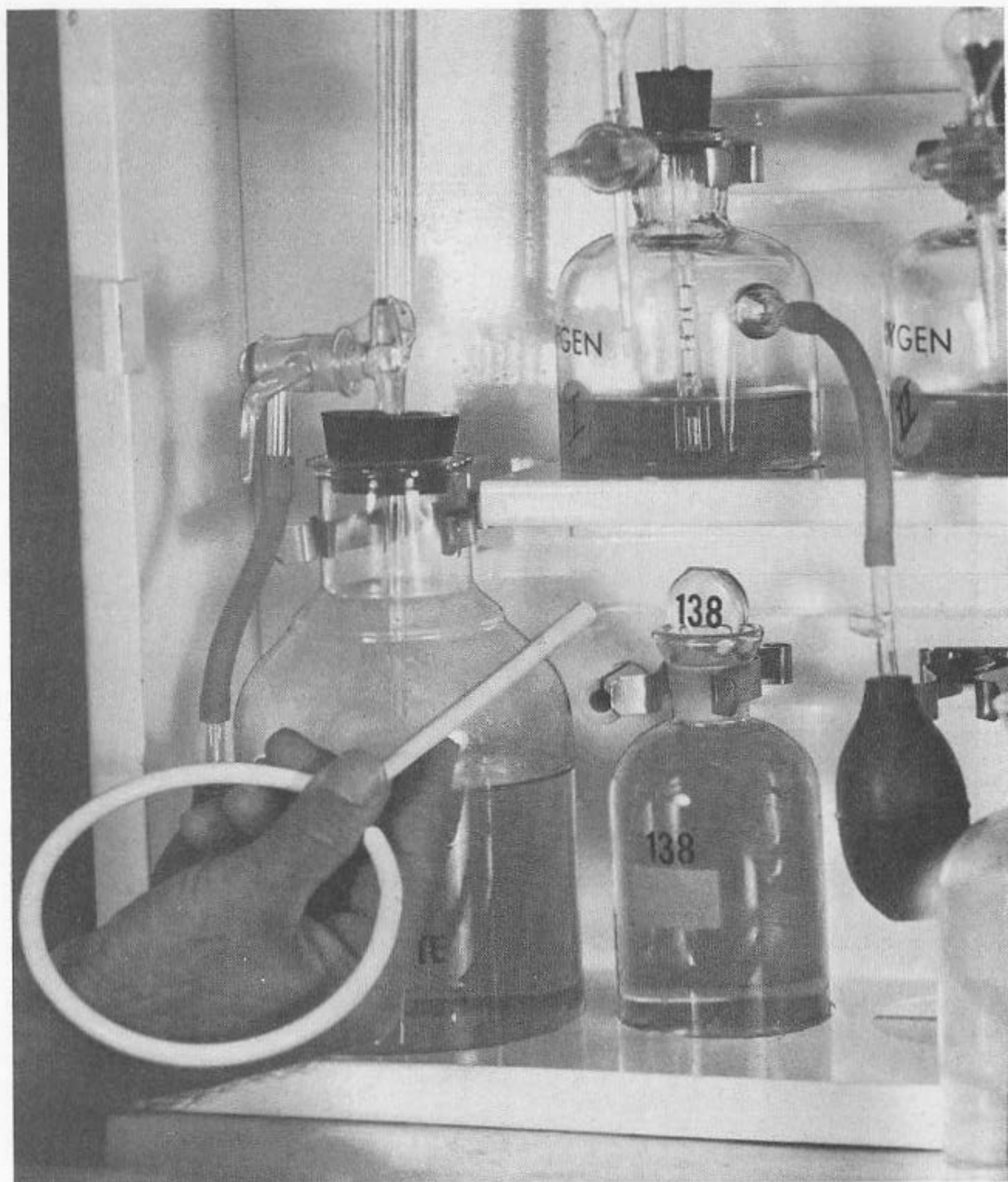
Figure 4-44.—Inserting iron ring in holder (dissolved oxygen test).
