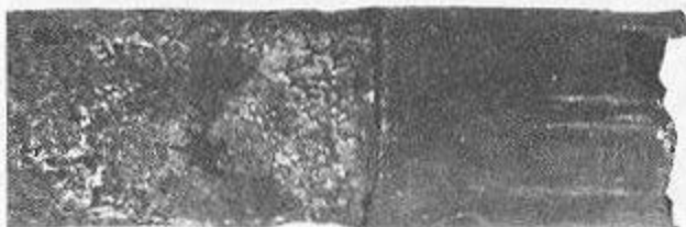
Figure 2-18.—General fireside thinning of generating tube.
