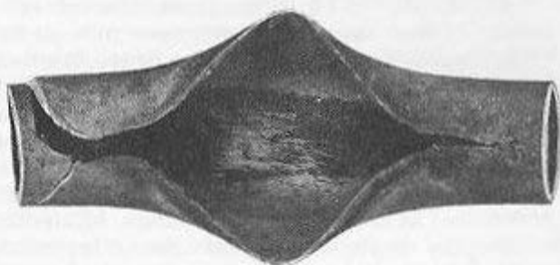
Figure 2-27.—Thick-lipped rupture in generating tube.
