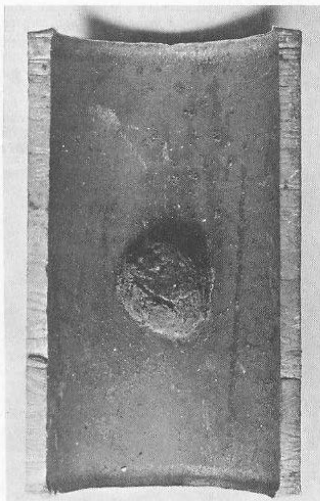
Figure 4-9.—Scab formed over oxygen pit.
