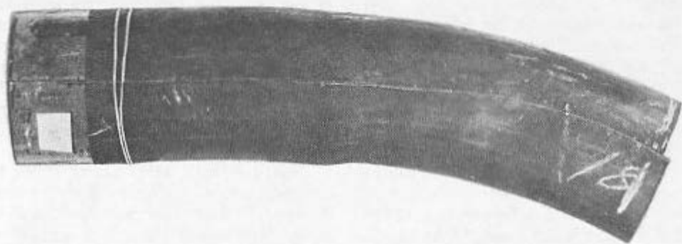
Figure 2-37. —Tube fold (fabrication defect).
