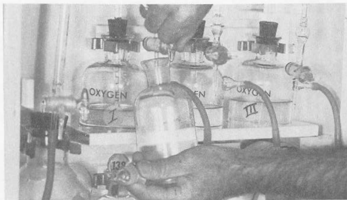
Figure 4-36.—Adding OXYGEN I solution to the sample (dissolved oxygen test).
