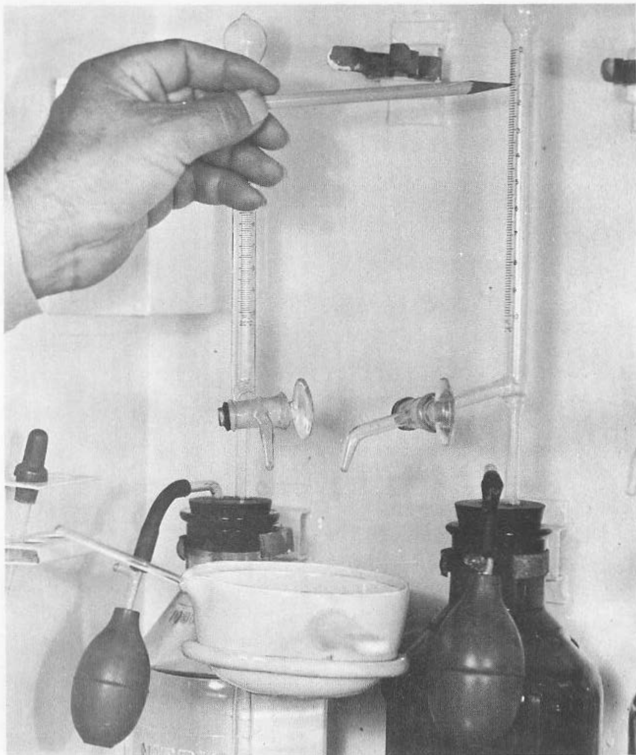
Figure 4-29.—Reading the burette (chloride test).
