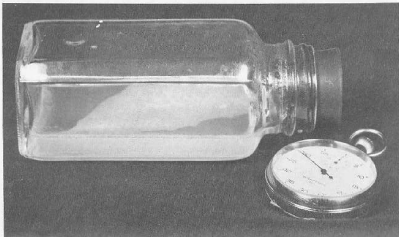
Figure 4-24.—Water is hard: Lather does not persist for 5 minutes over entire surface of sample.
