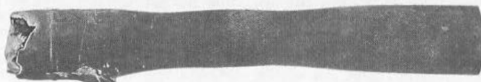
Figure 2-38.—Stretched or necked tube (fabrication defect).
