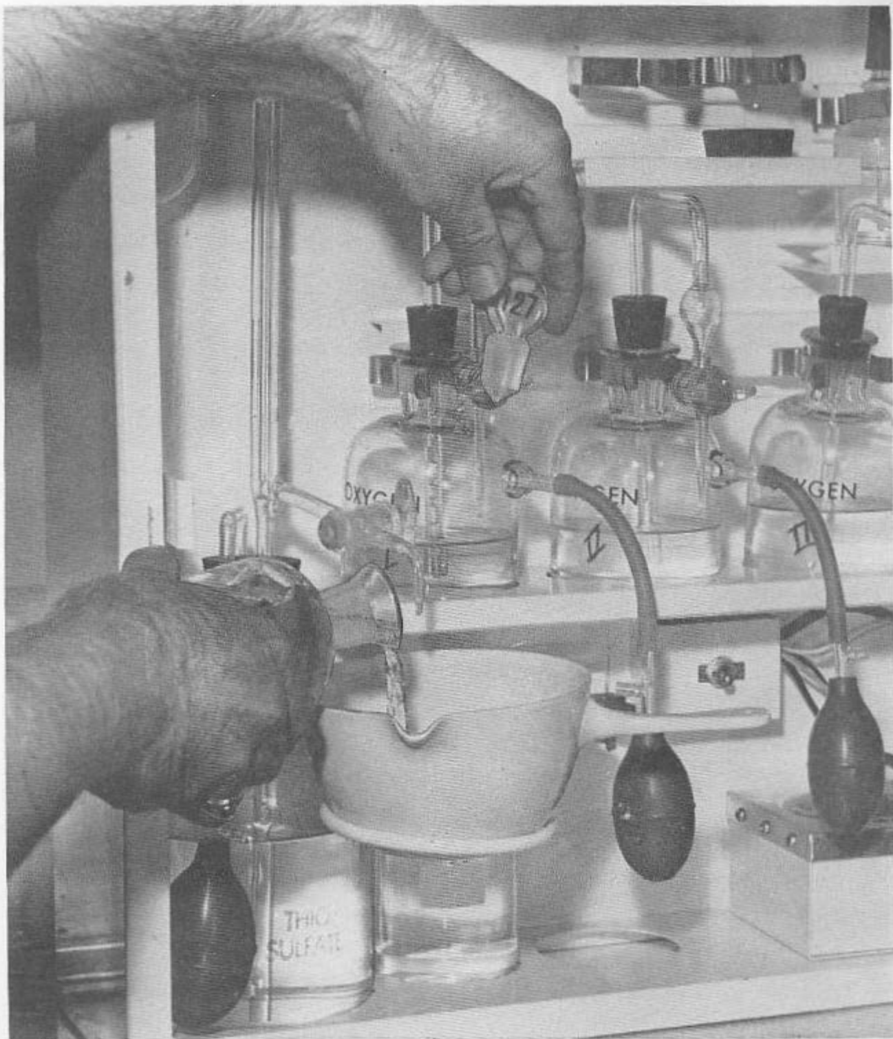
Figure 4-45.—Pouring the fixed sample into the casserole (dissolved oxygen test), 38.175
