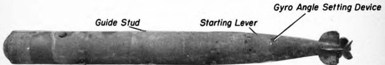
Figure 29—Type 44 torpedo with warhead removed.
