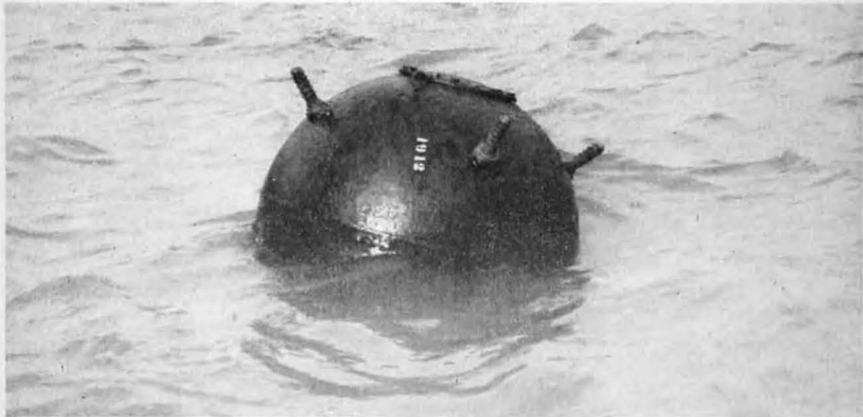
Figure 3—JA mine, floating, with its mooring cable cut.
