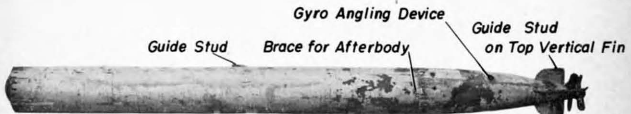
Figure 31—The 24-inch type 8th year long range torpedo with warhead removed.
