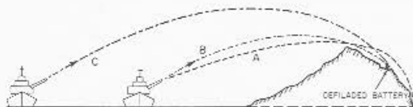
Figure 9-10. — Problem of hitting a defiladed target.
