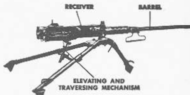
84.112 Figure 11-4.—Browning .50 caliber M2 machine gun (shown on the ground mount M3).
