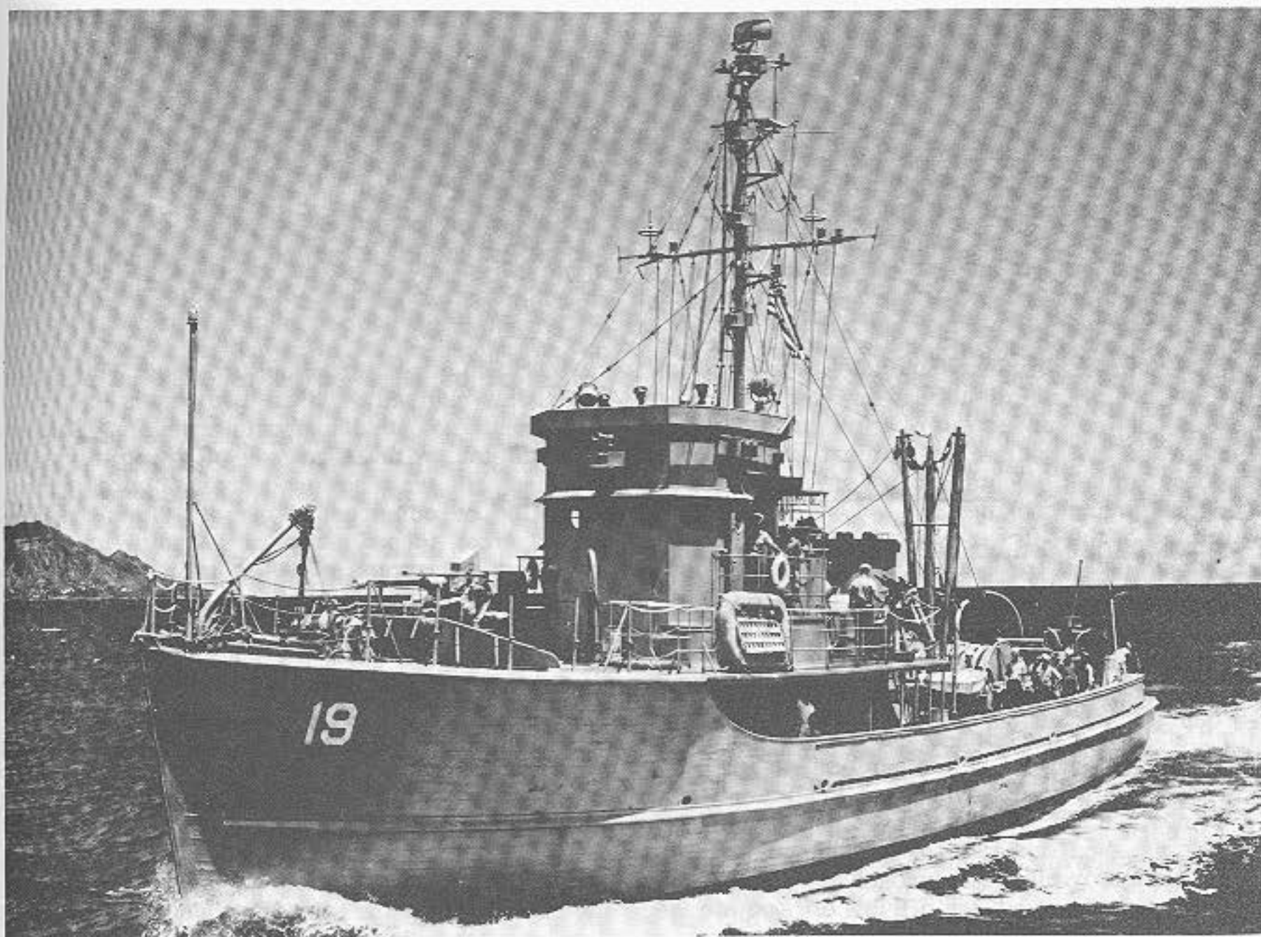
Figure 11-25.—Albatross class coastal minesweeper (old) has one 40 mm mount forward.
