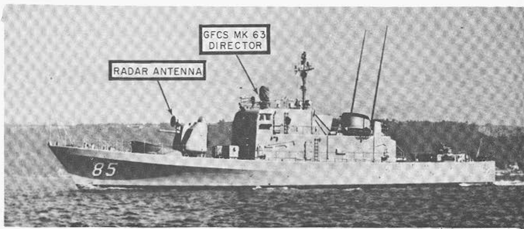
Figure 11-1.—USS Gallop (PG 85), an Ashville Class aluminum-hulled gunboat. She is armed with a 3-inch gun forward and a 40 mm gun aft, and her speed exceeds 33 knots.
