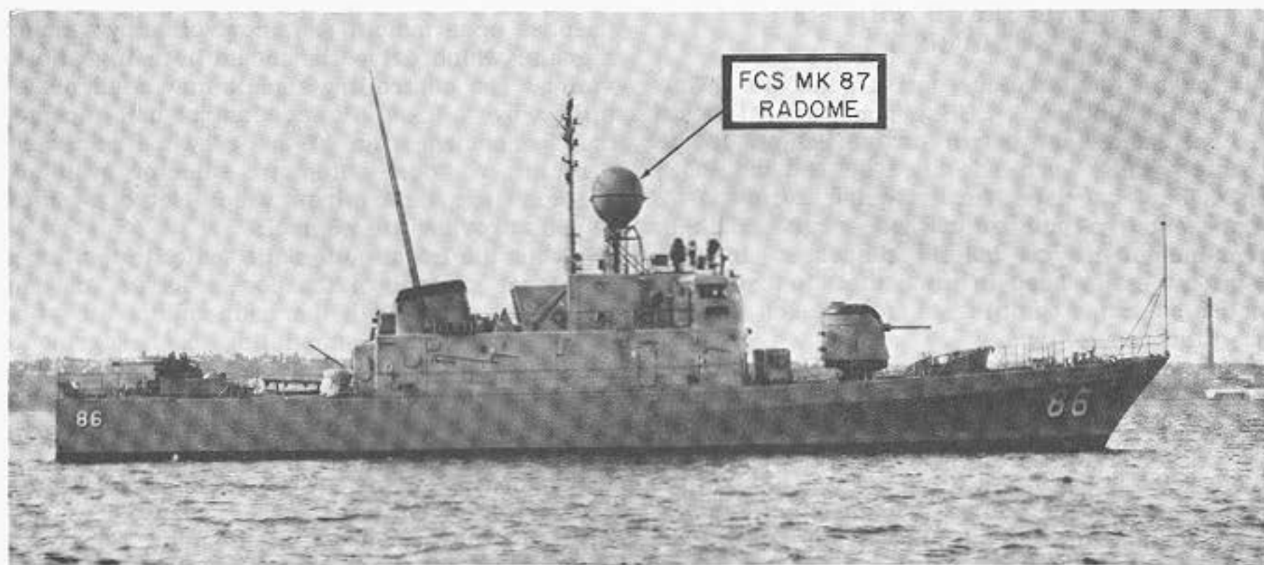
Figure 11-2.—USS Antelope (PG 86), with its FCS Mk 87 radome clearly visible above the pilot house.
