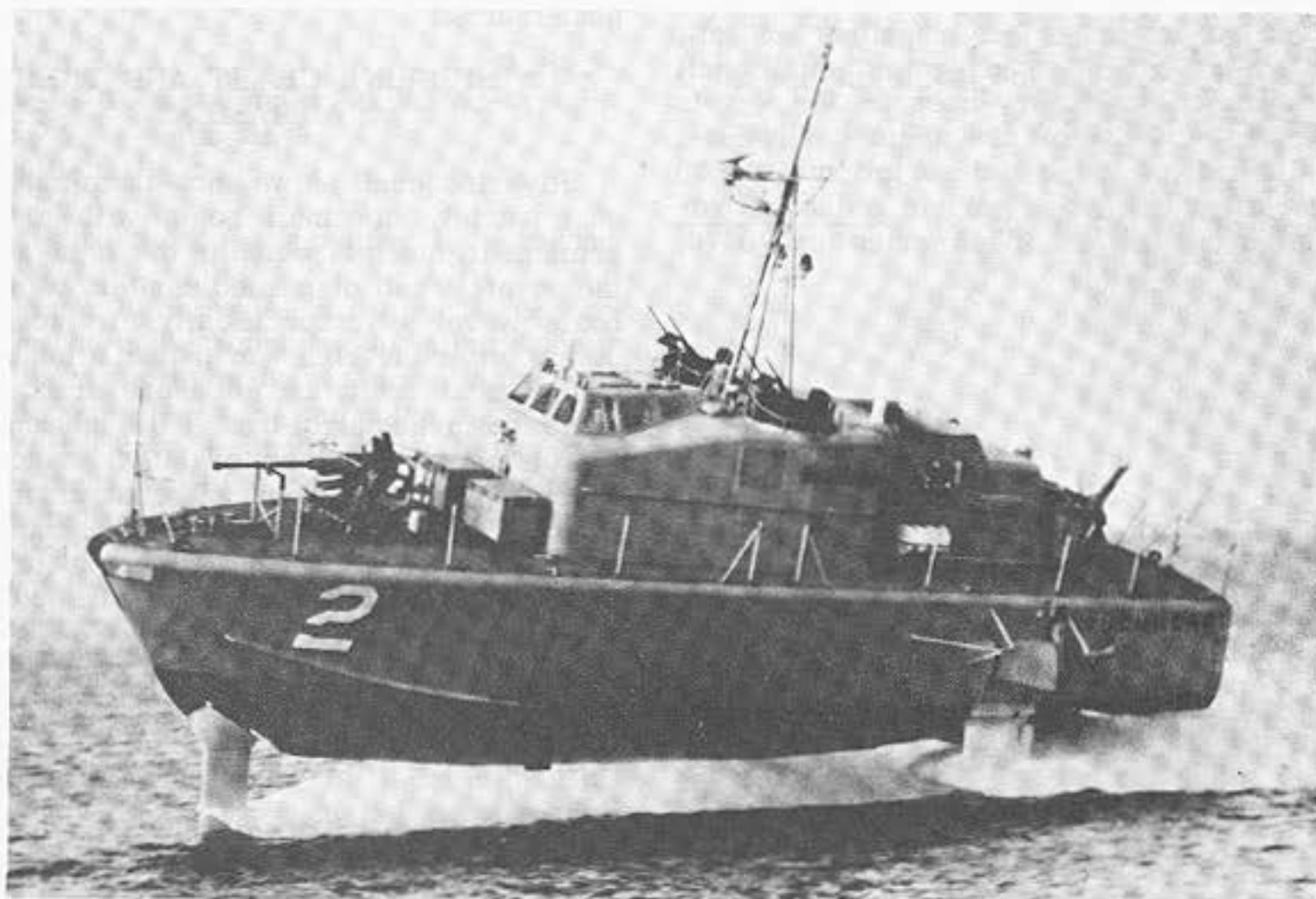
3.88(134) Figure 11-12.— Hydrofoil gunboat Tucumcari (PGH 2) with hydrofoils in the water.
