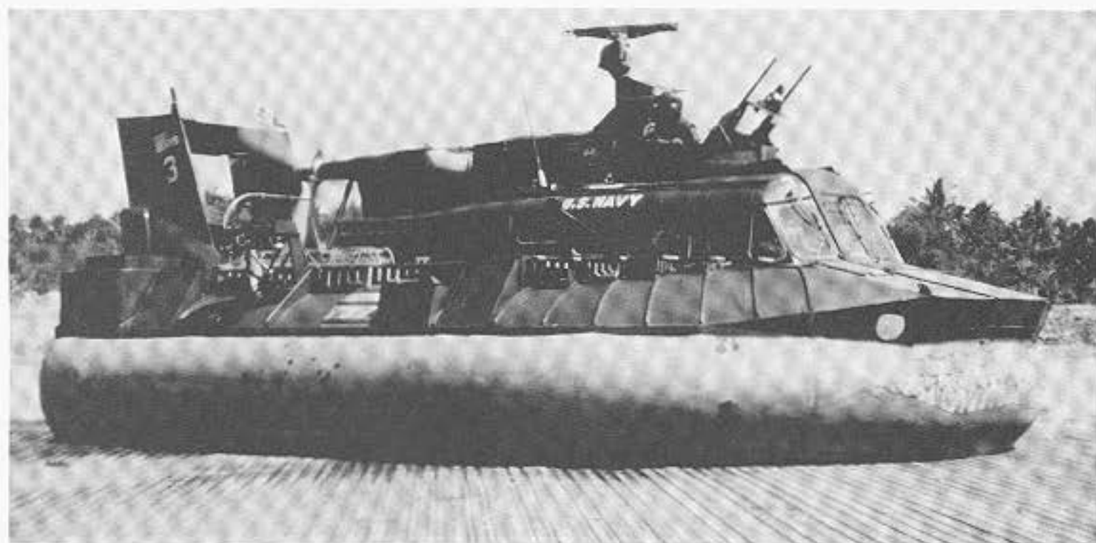
Figure 11-22.—The patrol air cushion vehicle, riding on a 4-foot cushion of air, can patrol or chase over any type of terrain.
